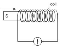
The needle of the galvanometer moves.
