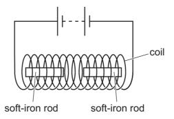
The connections from the battery to the coil are now reversed.
