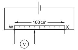
The potential difference (p.d.) between W and X is 1.5 V.
